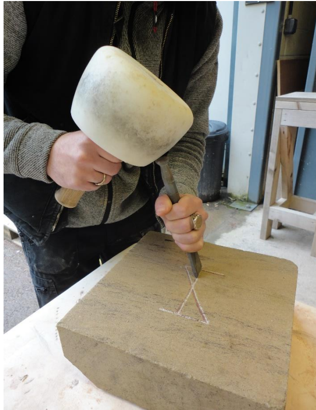
Figure 89: A mason demonstrates cutting a mason's mark
